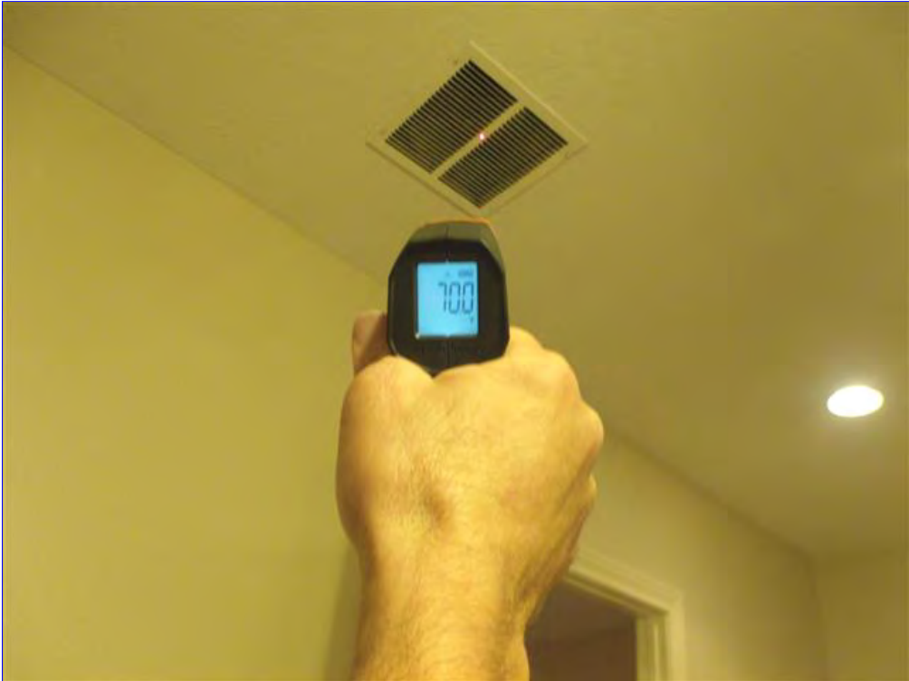
A. Item 1(Picture) Return vent 70° Air balanced OK
