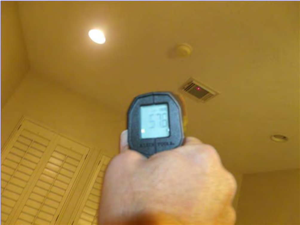
A. Item 2(Picture) Supply vent is 57.6°
